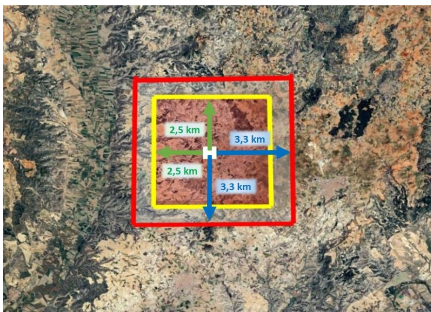
Illustration 17. Plan view of safety distances. Public-use civil heliports and military heliports.
